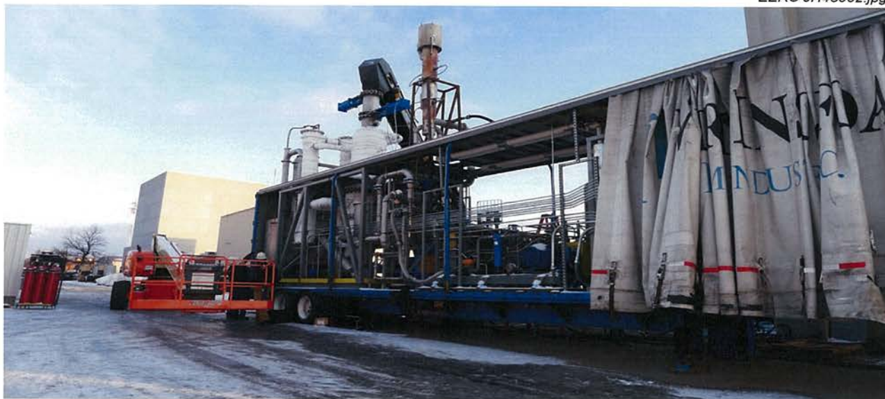
Figure 2. The completed MILS system. The gas-to-liquid reactor is behind the trailer curtain.
